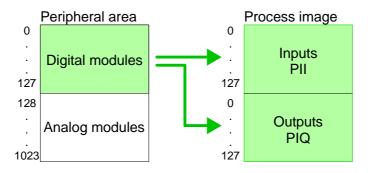
The process image is updated automatically when a cycle has been completed.
