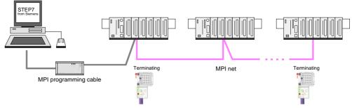
Transfer via Green Cable (serial communication)
